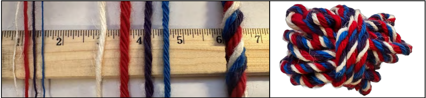
FIGURE 6.10 – Rashi yarn spun by the author. Left, Singles at 24-26 wpi. Middle, Six-ply yarn at 6-7 wpi, Right, 24-ply yarn at 3 wpi. Far right, small ball of 24-ply yarn. Linen spun using flax roving, wool yarns spun using pre-dyed merino wool.
