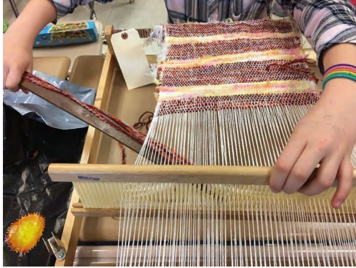
FIGURE 4.14– One of the author’s weaving students working on a modern rigid heddle loom. The student has lifted the heddle and is passing the shuttle between the two layers of warp strings. (Photograph from the Author’s collection.) (2019).
